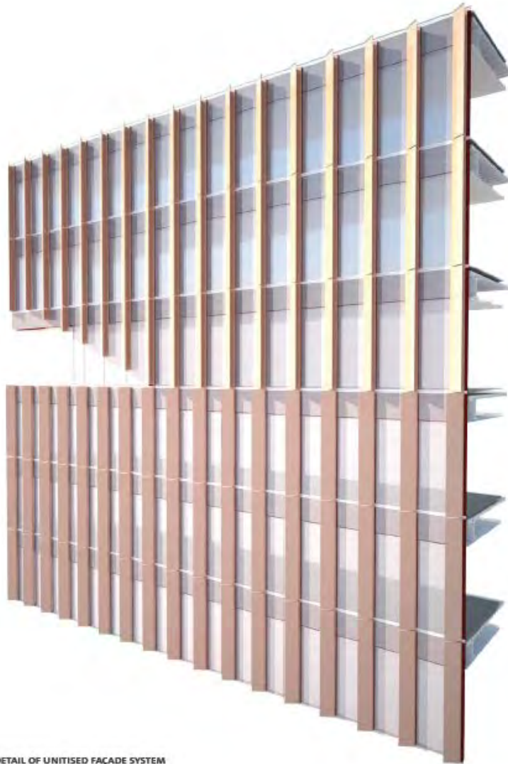
DETAIL OF UNITISED FAÇADE SYSTEM
